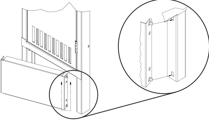
**2.** Rotate the front base into the left leg to lock in the locking tabs.
